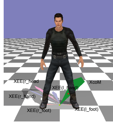
Figure 8. Index keys of a reactive motion. The appropriate reactive motion is searched for based on the eXtrapolated Center of Mass (XcoM) and the Extended End Effectors (XEE).
